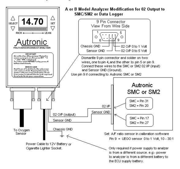
If connecting analyzer to Autronic SMC or SM2 always use Pin 9 (0 to 1 volt O/P) and select "UEGO sensor 0 to 1 volt, 10 - 30:1" in software, when using either a Bosch or UEGO sensor.
