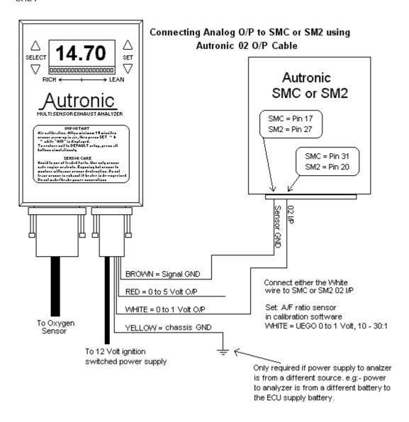
If connecting analyzer to Autronic SMC or SM2 always use WHITE wire (0 to 1 volt O/P) and select "UEGO sensor 0 to 1 volt, 10 - 30:1" in software, when using either a Bosch or UEGO sensor.
